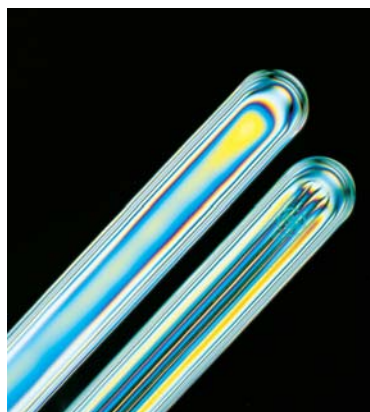
Klinger transparent glass (left side) and reflex glass (right) in polarized light
